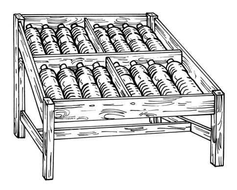
Solar disinfection (SODIS) with plastic PET bottle placed in the sun is an easy way for classes to make drinking water safe. Here is a SODIS stand that parents built. After 6 hours in the sun, the water is safe to drink.
