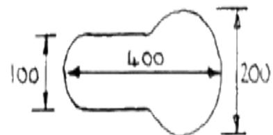
Raised foot pads to either side of the squat hole help keep feet and shoes hygienic and clean. If pouring a cement sanitation platform, these footpads should be built into the design. If making a more “do it yourself” latrine and platform, flat rocks can serve as adequate footpads. Be sure to anchor them firmly in the dirt floor.
