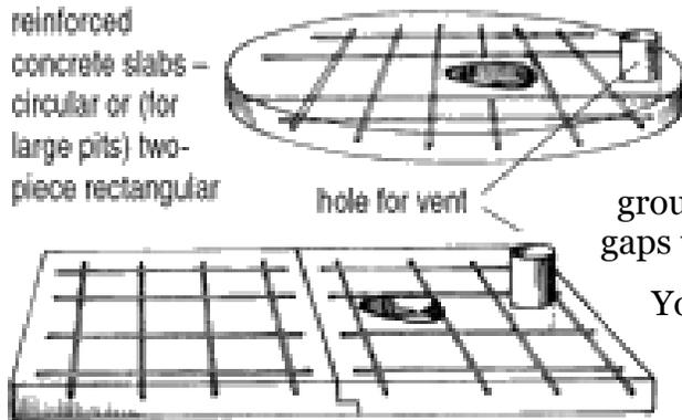
The size of the slab can be the same size as the outer lining if this is built of brick. If the lining is made from an oil drum or basketwork it needs to be slightly larger so that at least 200mm of the slab rests on the ground all round the pit. There should not be any gaps under the slab to let flies or smells leave the pit.
