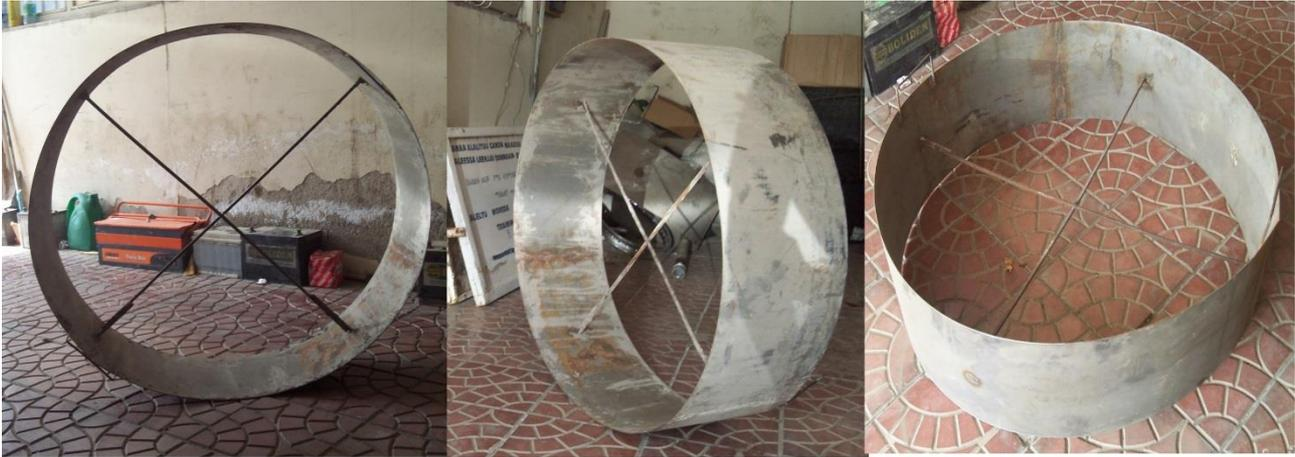
Figure 5: mold for pit lining
