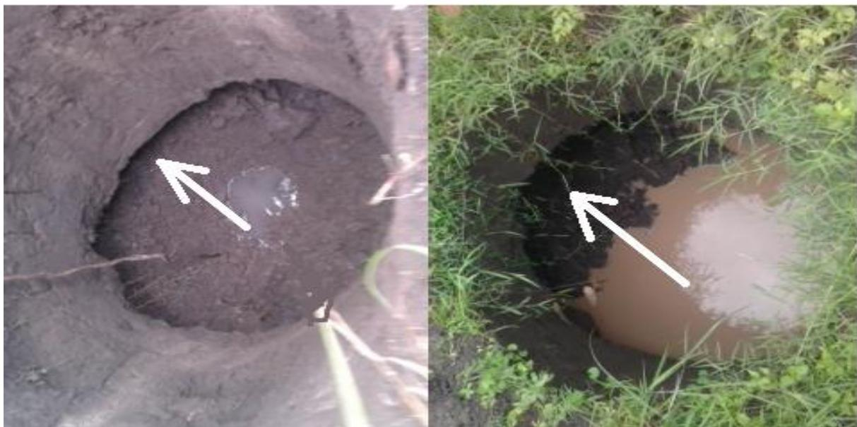
Figure 2: How pit collapse happens
