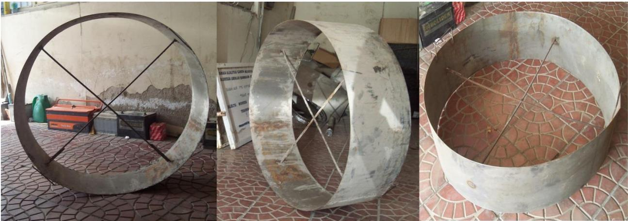
Figure 5: mold for pit lining
