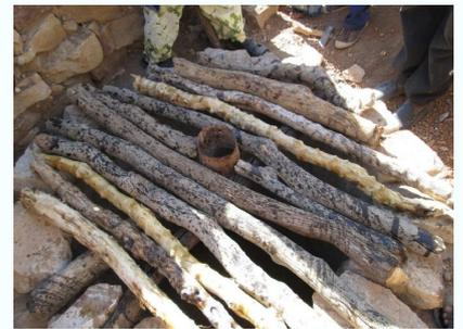
3. The wood is coated with engine oil to resist termite attacks.
